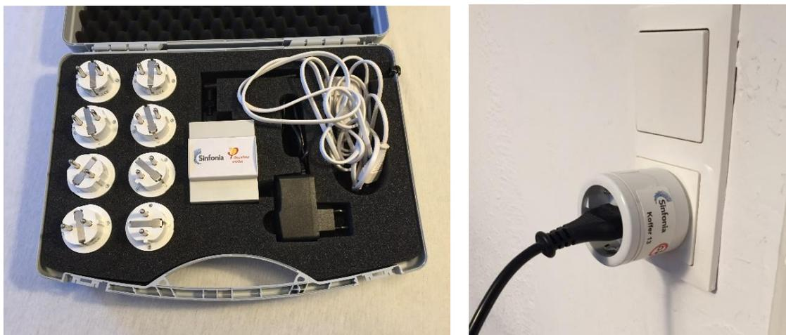
**FIGURE 1: LEFT: DATA ACQUISITION SET COMPRISING SMART PLUGS AND SINGLE BOARD COMPUTER, RIGHT: SMART PLUG IN USE**
